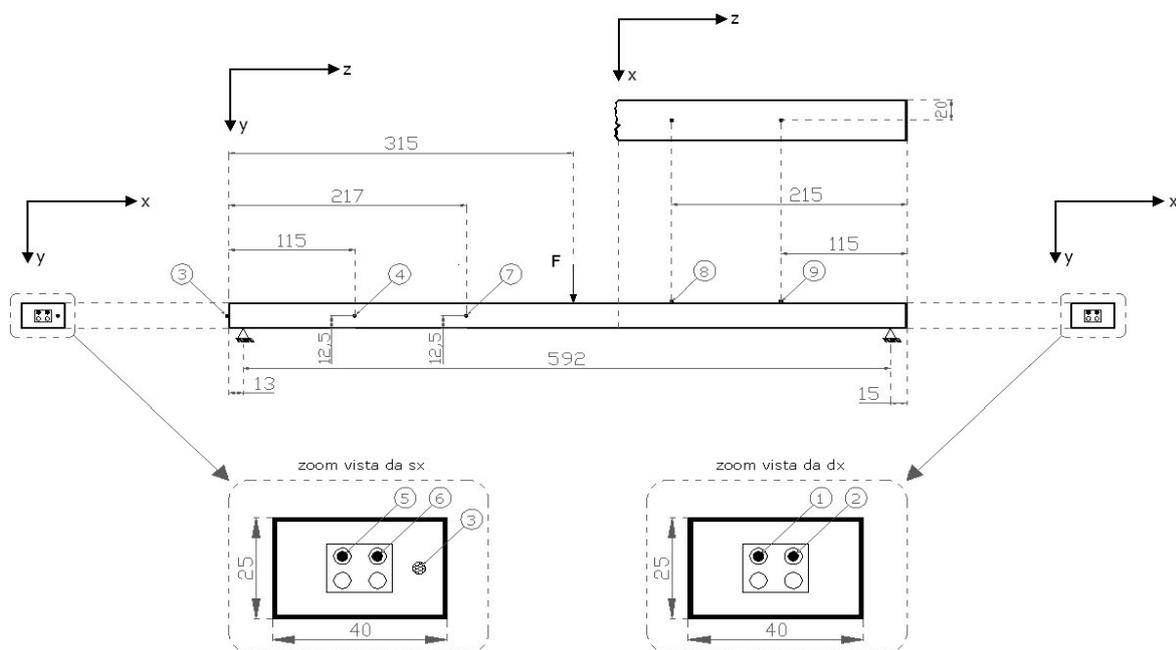
Figure 2. Side view and lateral view of the beam in the three point bending test condition. Circled numbers refer to sensor location.
