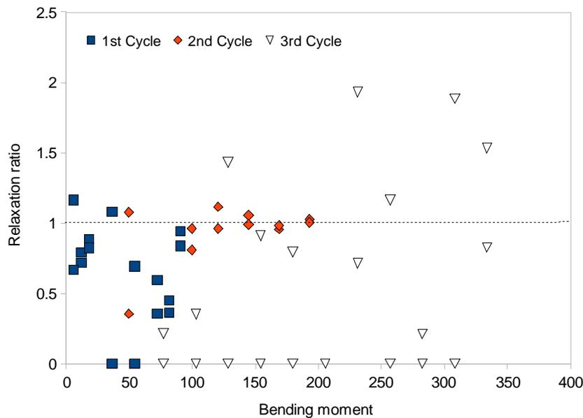
Figure 8. Relaxation ratio vs. bending moment during loading cycles
