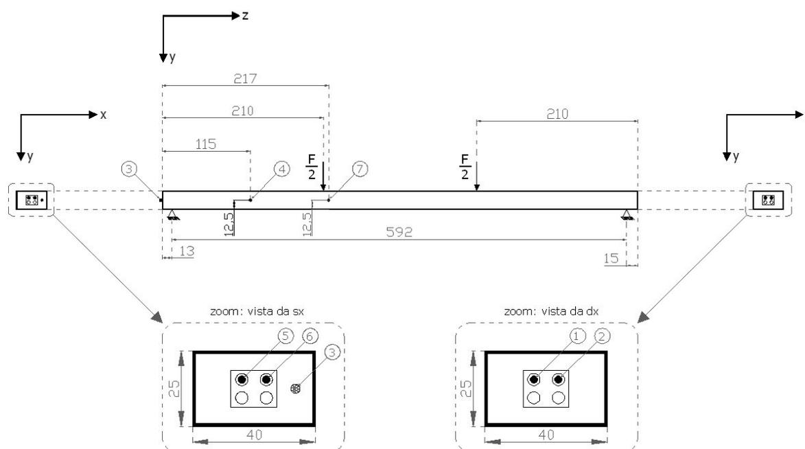
Figure 1. Side view and lateral view of the beam in the four point bending test condition. Circled numbers refer to sensor location.
