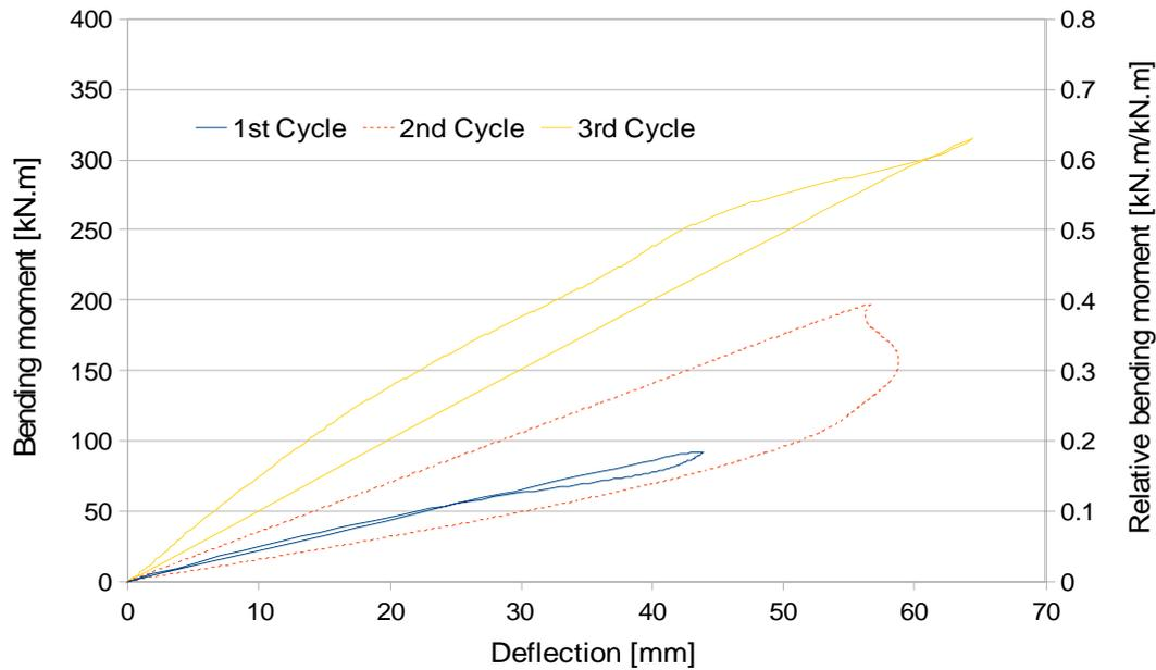
Figure 4. Bending moment vs deflection for the three loading cycles. Relative bending moment was calculated respect to the theoretical bending moment to failure
