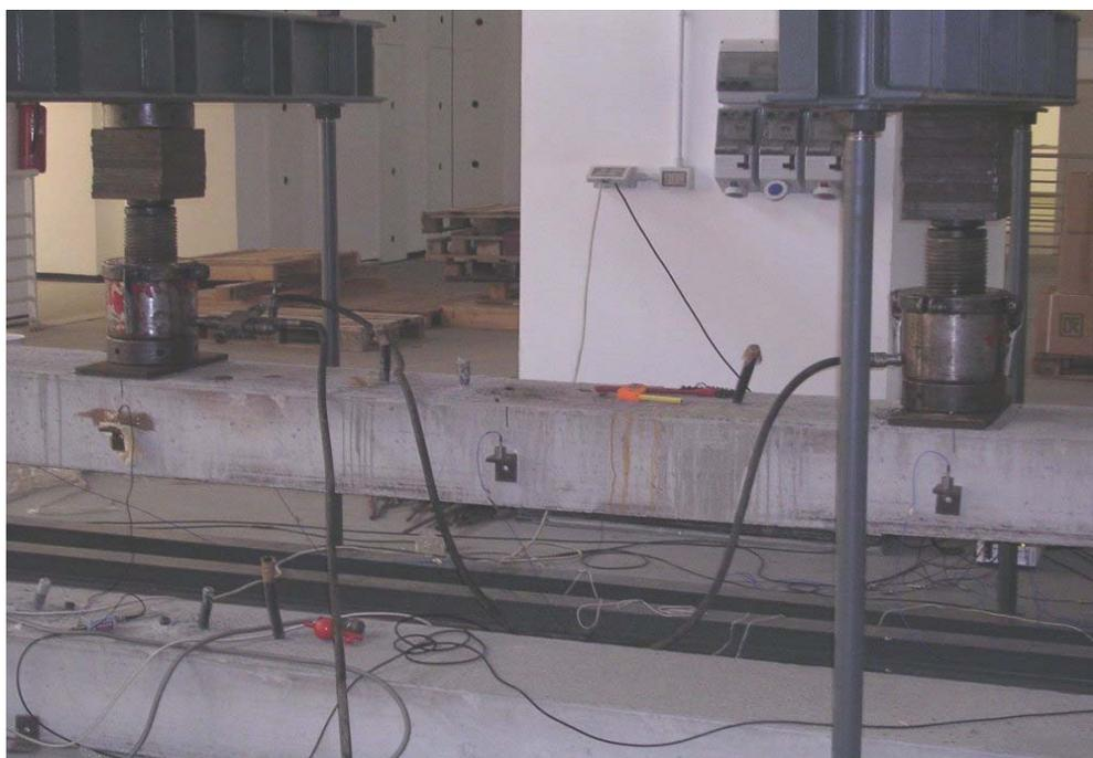
Figure 3. Four point bending test set-up
