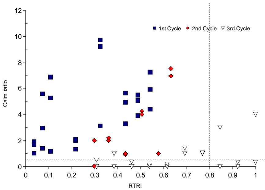
Figure 6. Calm ratio vs. RTRI ratio during loading cycles
