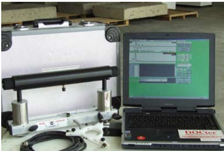
Figura 10 - Impact Echo test system
